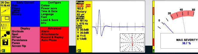
Meter display with alarm box being used to detect and evaluate defects.
